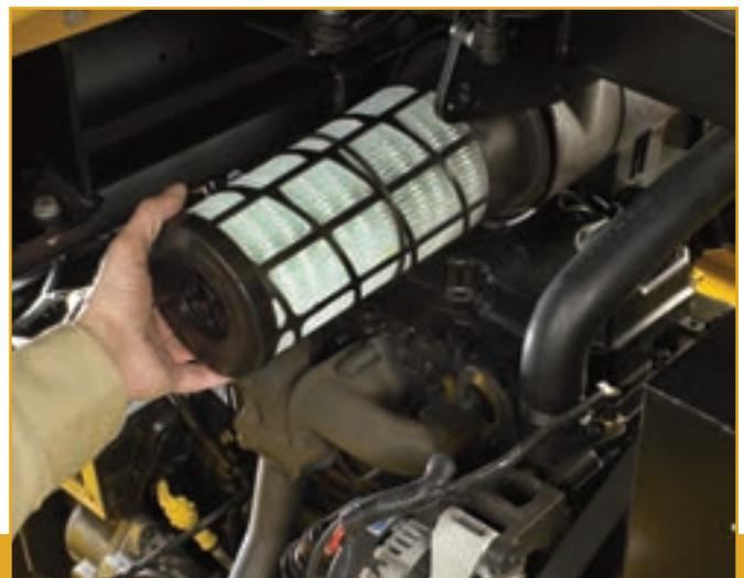
The Veracitor® VX truck features gas-spring assisted, gull-wing design engine covers. Coupled with the one-piece floor plate, it provides **excellent access**. Easy to remove floor plate requires no tools and gull-wing engine covers offer complete access to the powertrain. Engine compartment daily checks are all located within close reach and are easily performed. The uncluttered layout under the hood offers **clean hydraulic and electrical routings**.
