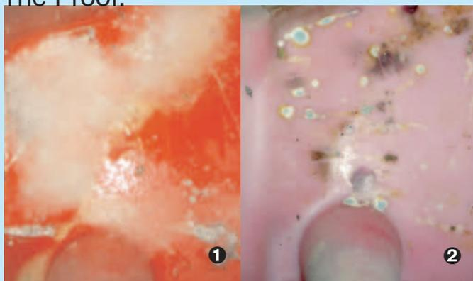
Two prepared tanks ① without AntiBac ② with AntiBac were closed and stored at room temperature for 7 days. After this time in the Hako AntiBac tank there is considerably less growth of bacteria, mould and spores. The Hako AntiBac tank also develops significantly less unpleasant smells.
