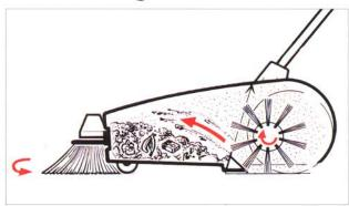
The side broom sweeps dust and debris from corners, directly into the path of the wide main broom, which in turn flips the same into the large self collecting hopper.
